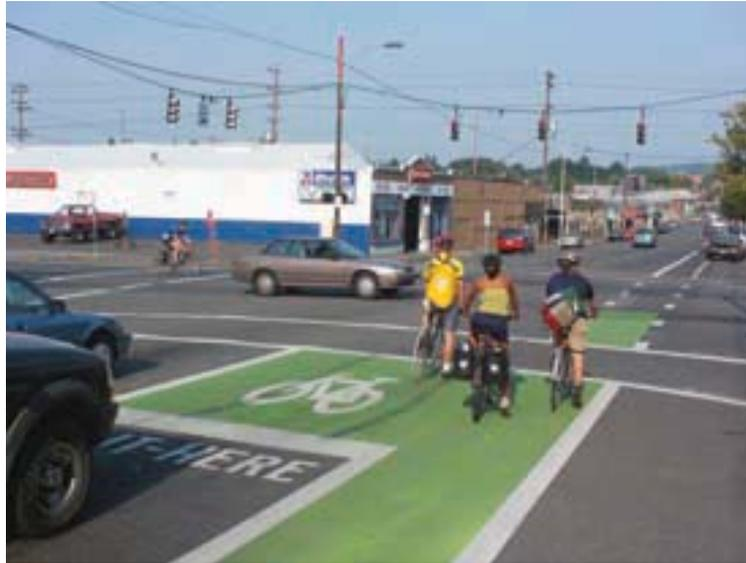
**Figure 7-8** By allowing cyclists to move in front of vehicles and by coloring the bike lane through the intersection, bike boxes create safer conditions for cyclists, particularly when drivers are planning to make right turns.
